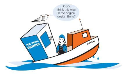
Keep an eye on how much extra weight you put on board your vessel as stores and equipment. Increases in weight take your vessel lower in the water, limiting both its range of stability and the catch you can safely carry. The slow accumulation of stores and equipment over the years can end up making a big difference to how stable your vessel is. Think about having a clean-out, and always consider carefully where you are storing heavy items.
