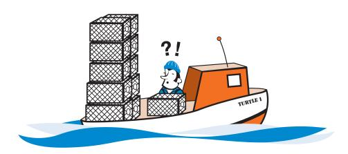
If you have a stability book, look at the 'loading conditions' prepared for your vessel. Loading conditions have been calculated for your vessel for specific amounts of fuel, stores and catch. Each scenario is designed to help you plan your trip and to highlight when the quantities of catch and/or fuel become a hazard. They should be thought of as useful guides to help you operate your vessel safely.
